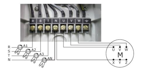
Current measurement: (see motor plate)
